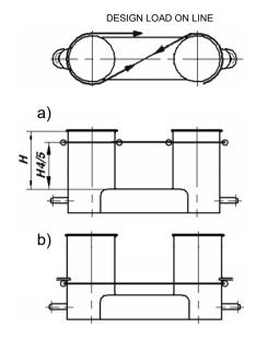
4.5.3 Under the design load conditions, as specified in 4.3, the allowable normal stress should be taken as 100% and the allowable shearing stress as 60% of the specified yield point for the material used. Normal stress is the sum of bending stress and axial stress with the corresponding shearing stress acting perpendicular to the normal stress, no stress concentration factors being taken into account.
